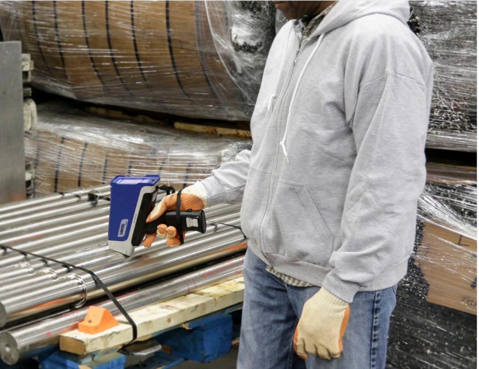
Olympus' new Vanta™ analyzer is our most advanced handheld X-ray fluorescence (XRF) device. These rugged, powerful, and intuitive instruments provide rapid, accurate element analysis and alloy identifications to customers who demand laboratory-quality results in the field.
