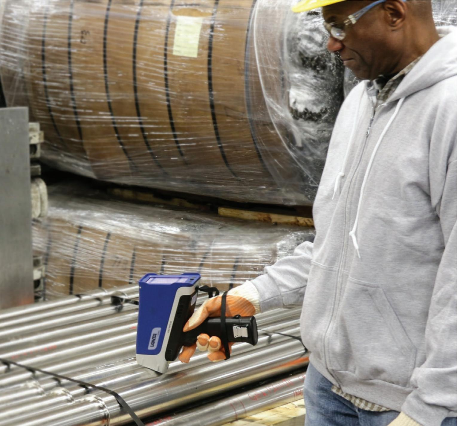
As the price of recycled metals fluctuates, identifying alloy grades quickly and easily is essential for profitability. Vanta™ handheld XRF analyzers for scrap sorting provide reliable identification in seconds for most alloys and pure metals.
