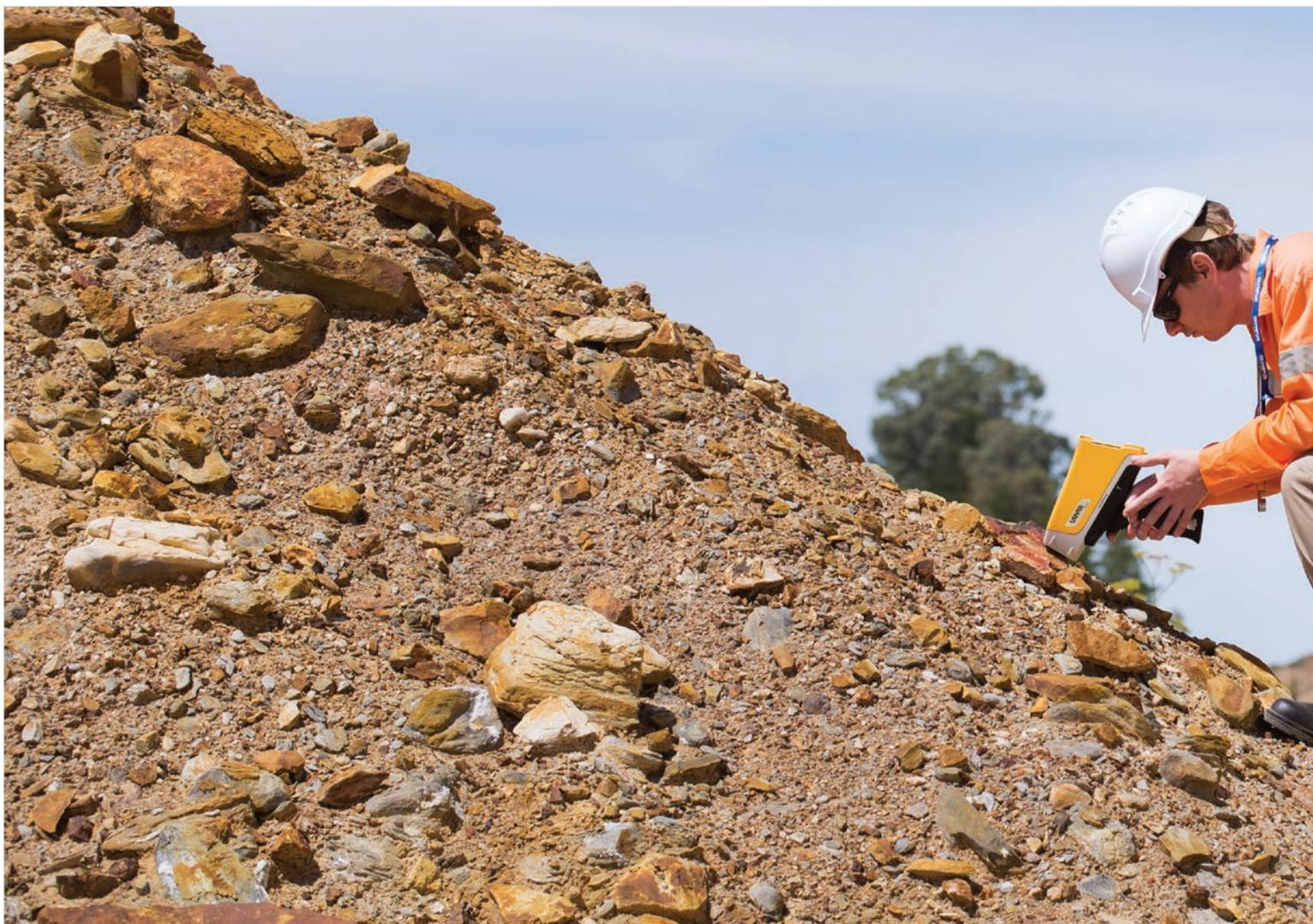
The Olympus Vanta™ handheld XRF provides immediate, on-site elemental measurements for a range of geochemical applications. Vanta analyzers provide power and flexibility across the entire mineral resource cycle:
